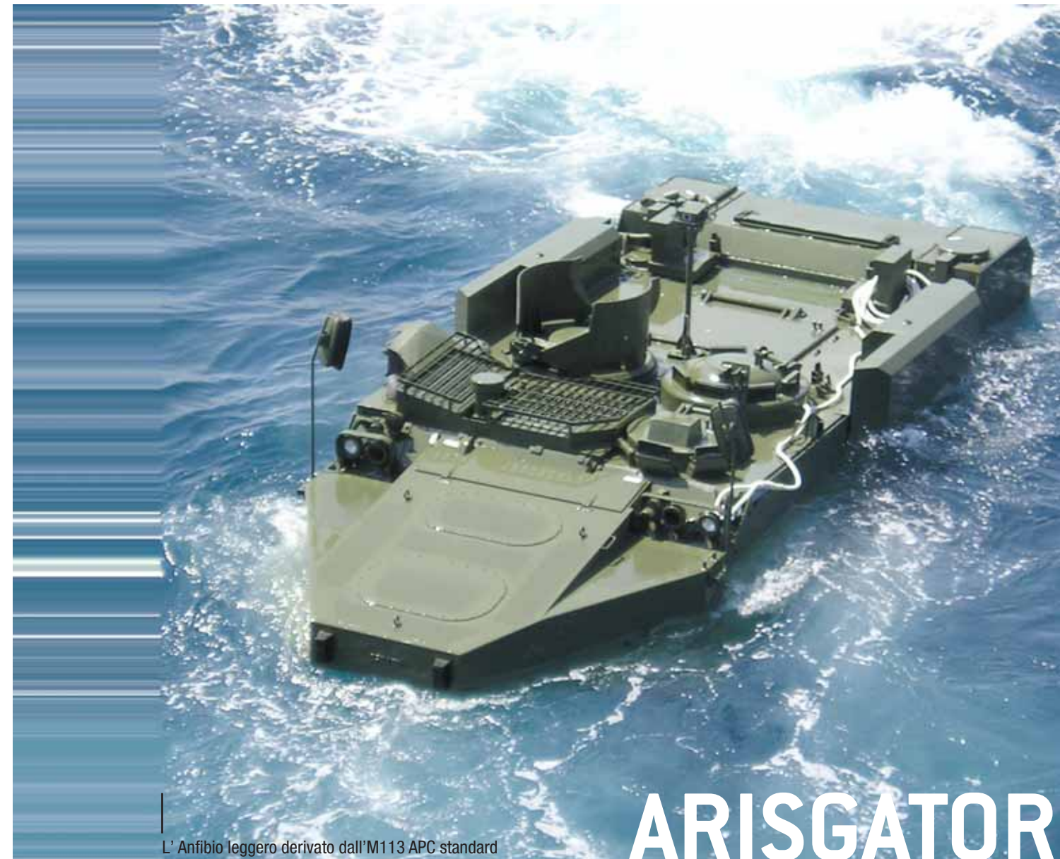
The light amphibious vehicle obtained from the standard M113 APC.
